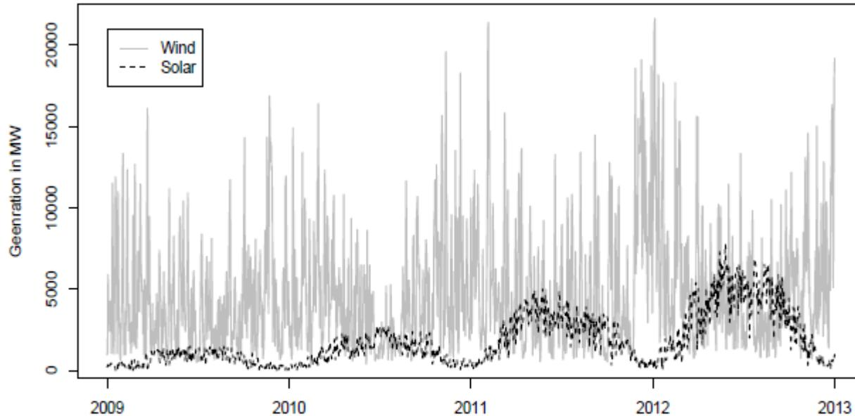
Figure 5: (Forecasted) Generation from Wind and Solar between 2009 and 2012
